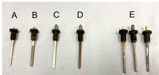
**Figure 4.** A photo showing the stages of Ag-rod refresh – (A) a rod ready for coating, (B) an undercoated electrode, (C) an unclean and/or stripped Ag rod where recoating has failed, (D) a correctly coated rod, and (E) a collection of degraded Ag rods after use.
