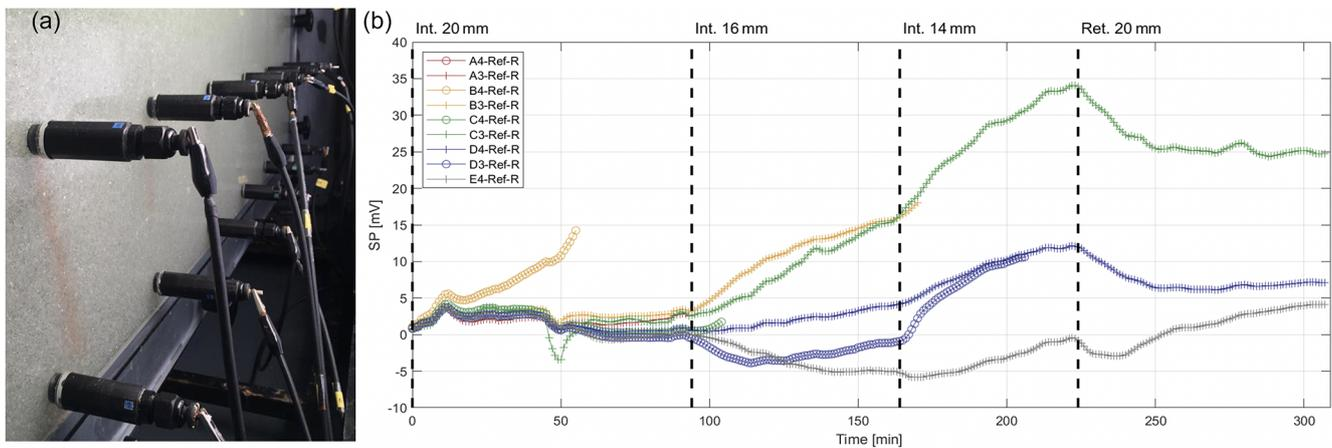
**Figure 10.** A photo **(a)** and recorded SP signals **(b)** from flush-mounted Electrode B examples made with 0.63 M “synthetic seawater” in a homogenous synthetic aquifer made of 1.09 mm silica beads, undergoing saline intrusion when synthetic seawater displaces “freshwater” and then retreats.
