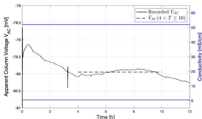
**Figure 8.** Results from a column experiment using the tap water and synthetic seawater electrolytes described in Table 2; two examples of Electrode B were assembled using synthetic seawater. The figure shows the recorded apparent column voltage recorded against time; also plotted is mean voltage from  $t = 4$  to 10 h as a dashed line. The right-hand axis shows the conductivities at the top and bottom of the column (in blue).
