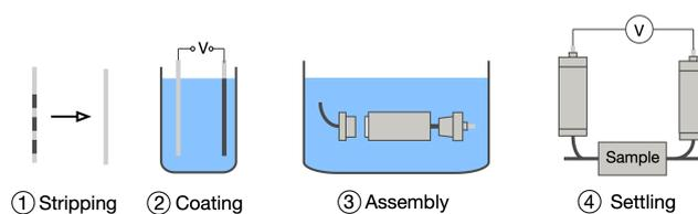
**Figure 3.** The four stages of electrode preparation.
