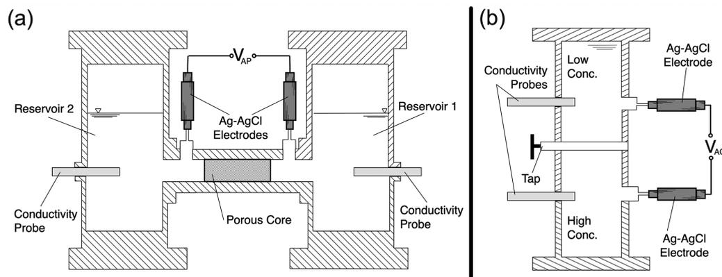
**Figure 6.** Cross-sectional sketches of the apparatus used to measure the exclusion–diffusion potential across a saturated sample (a “plug”). Panel (a) shows the “plug apparatus” for measuring the exclusion–diffusion potential across the sample; panel (b) shows the “column apparatus” for measuring the diffusion potential across the two electrolytes of interest.
