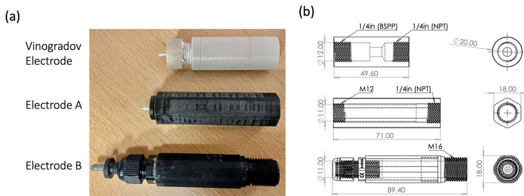
**Figure 2.** A photo (a) and major dimensions (in descending order) of the Vinogradov electrode, Electrode A, and Electrode B (b).
