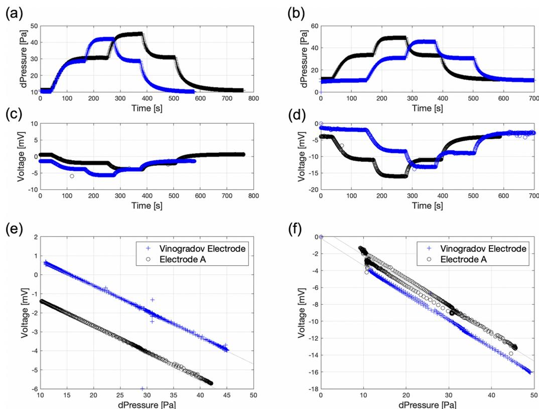
**Figure 7.** Streaming potential results for the glass beads obtained using synthetic seawater (a, c, e) and tap water (b, d, f) comparing results from the VE and the developed Electrode A. Plots (a) and (b) show pressure change over time, plots (c) and (d) show voltage change over time, and plots (e) and (f) show stabilized voltage against stabilized pressure drop.
