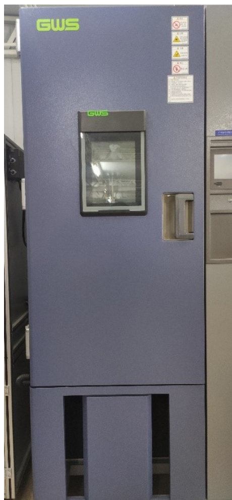
Figure 5. The programmable air bath.
