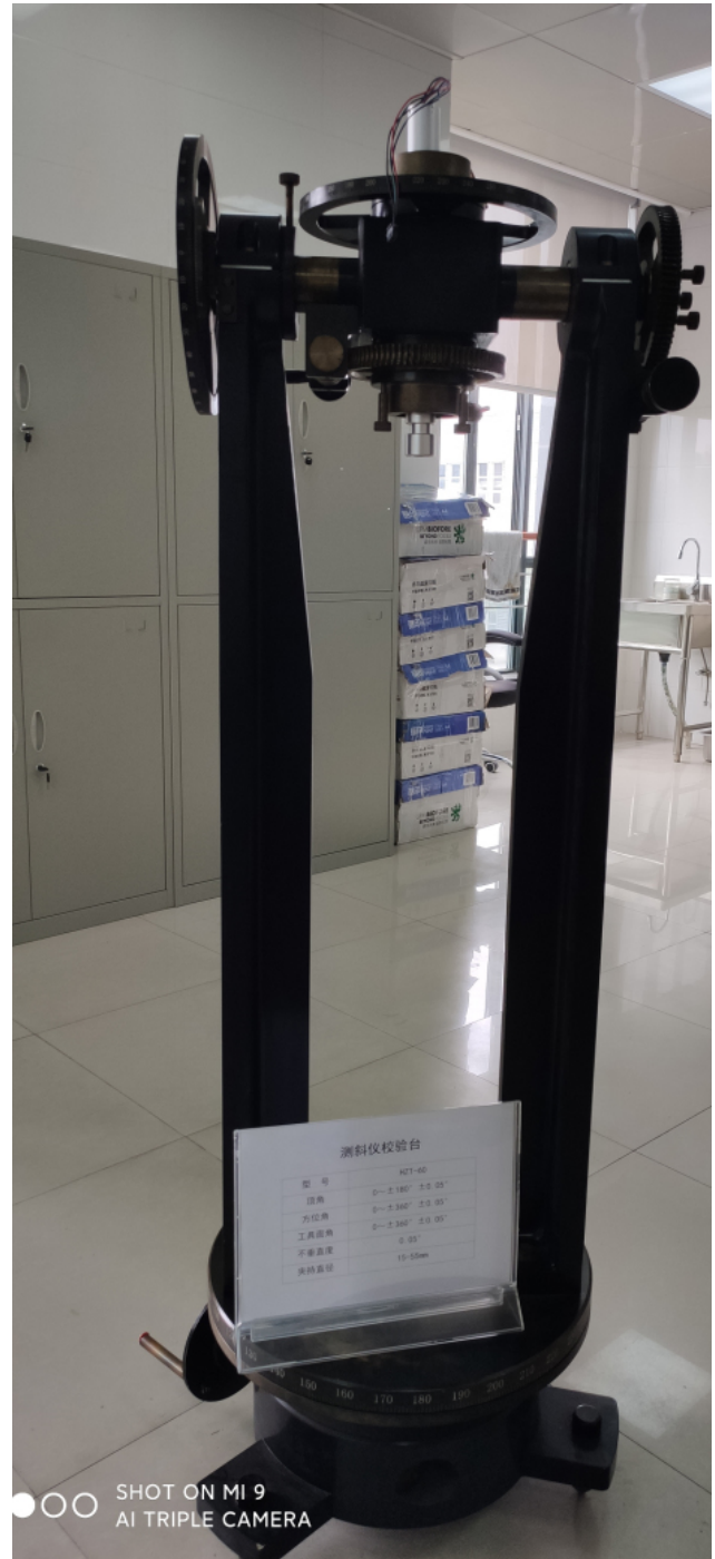
Figure 8. HZT-60 inclinometer calibration table.
