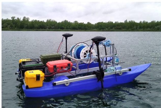
Figure 1. An expanded implementation of the MARP-FG concept supports a payload capacity of 100 kg. This enables the platform to carry an ultrasound scanning system or, shown here, a winch with a multisensor probe capable of descending to depths of up to 70 m water depth. The thrusters are Minn Kota electric drives.
