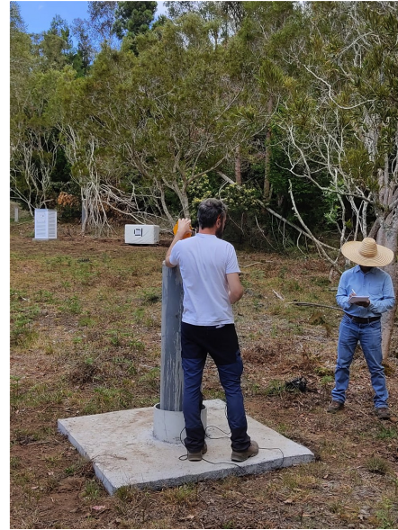
Figure 2. Left: a schematic map of the observatory. Right: photograph showing the layout of the La Réunion Observatory. In the foreground, the main observatory pillar is seen during a training session. In the background, from left to right, are the grey concrete target pole; the white meteorological box housing the sensor electronics; the grey vertical PVC tube, partially obscured by trees, containing the variation scalar magnetometer; and the plastic box containing the variation vector magnetometer, covered with a white thermal blanket.
