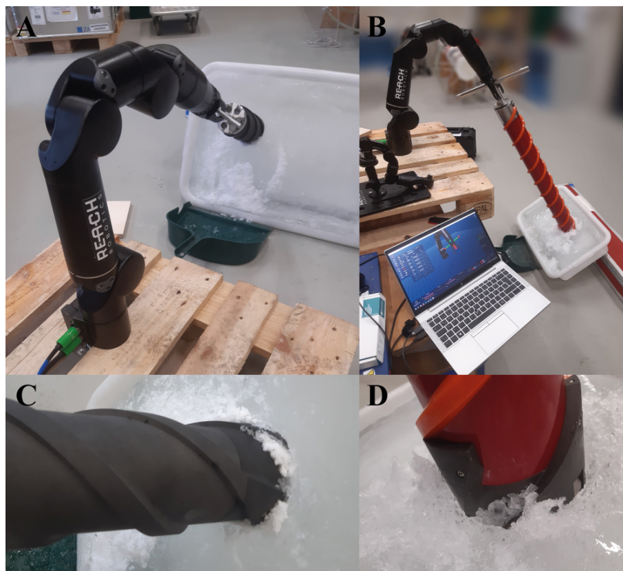
Figure 1. Experimental ice drilling setup. The manipulator arm is mounted to a wooden pallet for both coring systems. (a) and (c) show the self-constructed short ice corer, while (b) and (d) show the setup using the commercially available Kovacs Mark II coring system. (b) shows the control laptop running the “Reach Control” software as well as the pendant master arm controller just in front of the manipulator arm.
