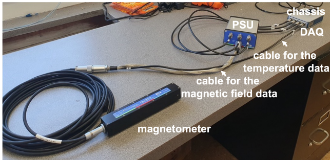
Figure 1. The elements comprising the instrumentation system of our geomagnetic variometer station, assembled in our lab. The magnetometer is a three-axes fluxgate Bartington Instruments magnetometer and is powered by a Bartington Instruments power supply unit (PSU). The data acquisition module (DAQ) is a NI-9239 from National Instruments, which contains an analog-to-digital converter. The output digital data are collected by a NI cDAQ-9171 (chassis), which is connected via USB to a mini PC by Intel (not shown here). See text for more details.
