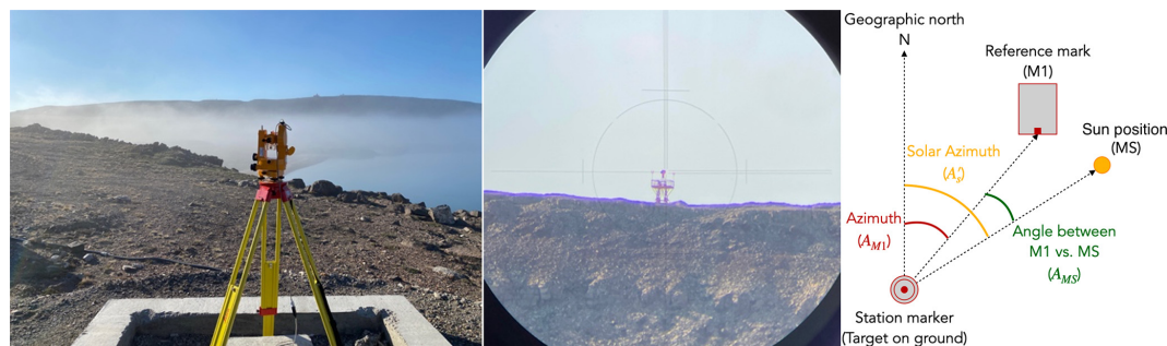
Figure 3. Sun observations for azimuth determination. Left: The fluxgate theodolite mounted above the Pillar A foundation at PIF, aligned toward a distant reference mark located several kilometres away. Centre: View of the reference mark (M1) through the theodolite's monocular. Right: Illustration (by Marie V. Eldor) showing the key angles involved in a sun observation. A_{M1} is the essential azimuth angle for accurate declination measurements.
