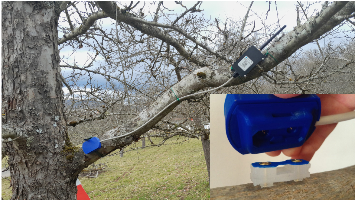
Figure 5. Example of a TreeSense Pulse sensor (blue box) connected to telemetry unit on an apple tree located in an orchard meadow and embedded electrodes, screwed into a tree branch, and sensor cover with connectors to the telemetry module.
