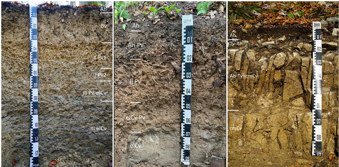
Figure 4. Soil profiles at Sites 1 (left), 2 (middle), and 3 (right). The German soil classification guide (AG Boden, 2024) was used for soil description, and soil classification was done according to the World Reference Base for Soil Resources (WRB) classification system (IUSS Working Group WRB, 2022).
