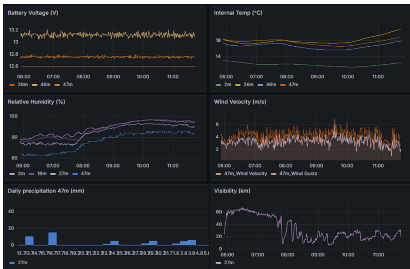
Figure 5. Screenshot of Grafana dashboard showing data from weather stations installed on the above-canopy tower.
