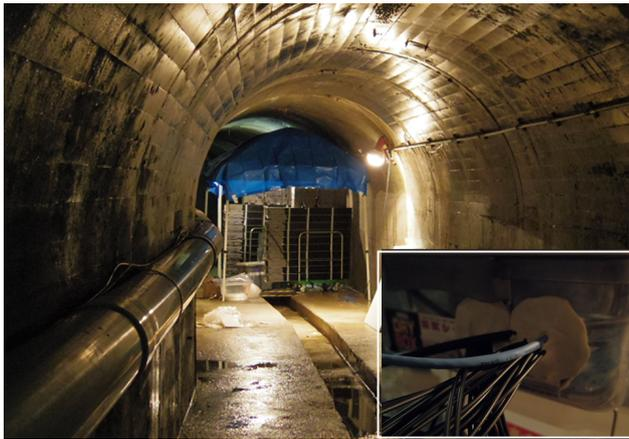
Fig. 6. Photograph of the muon radiography measurement system in the drain tunnel and a housing of the muon readout module (inset).
