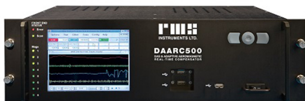
Figure 9. RMS DAARC500 compensation system (source: modified from RMS 2015, http://www.rmsinst.com/images/DAARC500.jpg , last access: November 2015).
