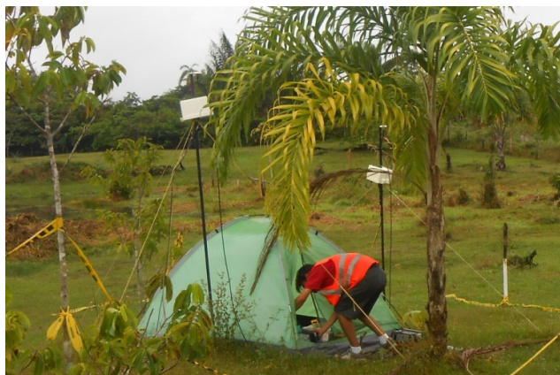
Figure 15. Example of a day monitoring BaseMag station, which measures the magnetic field in parallel to an airborne geophysical acquisition site (source: S. Guimarães, author private collection, January 2015).
