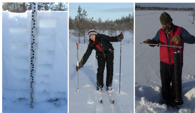
Figure 2. Different methods utilized for snow depth and SWE measurements during the SnowSAR-2 campaign. Conventional snow probe (left), Magnaprobe (middle), and SWE coring tube (right).
