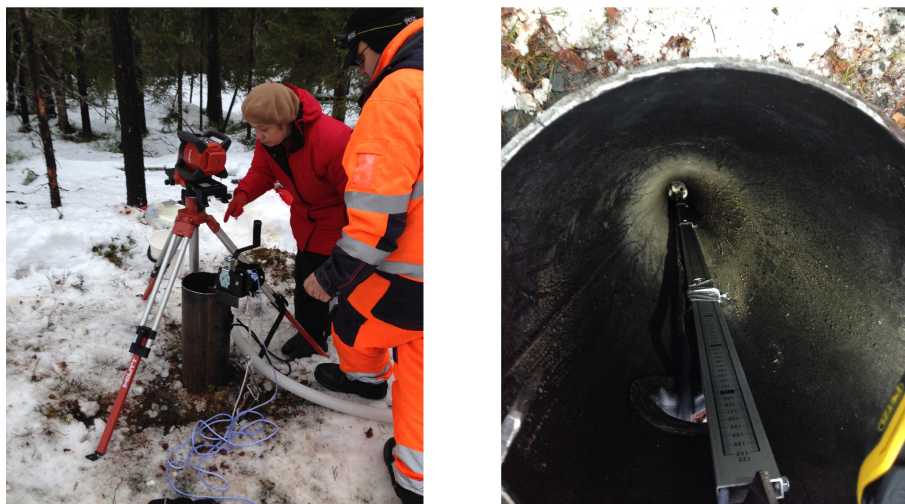
Figure 11. Installation of the Trillium Posthole 120PH seismometer in a drill core of depth of 5.5 m at the Oulanka site (station code OLKF). Photo by Hanna Silvennoinen.
