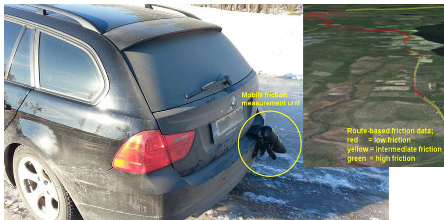
Figure 6. Teconer friction measurement instrument mounted onto the vehicle.
