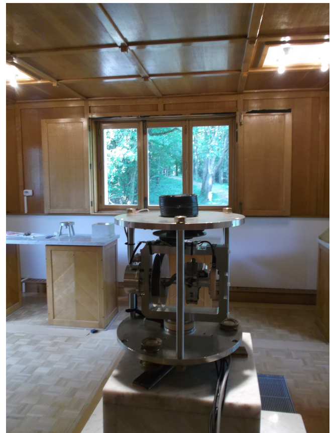
Figure 4. AutoDIF mk2.2 on pillar DO2 in Dourbes absolute house.
