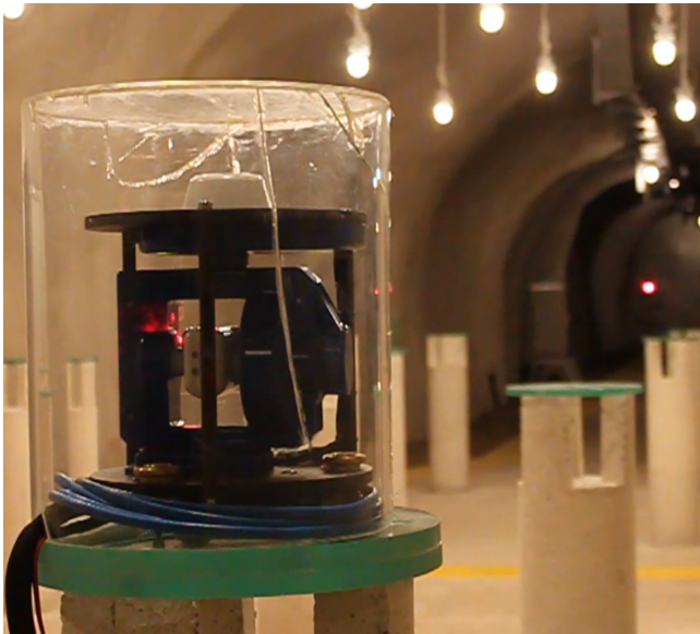
Figure 6. AutoDIF mk2.2 with its Plexiglas cloche on pillar A16 in the tunnel of Conrad observatory (WIC).
