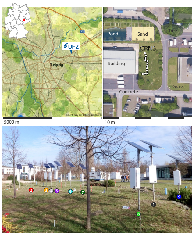
Figure 2. Location and arrangement of the nine cosmic-ray neutron sensors deployed at the small, urban meadow at UFZ Leipzig, Germany.
