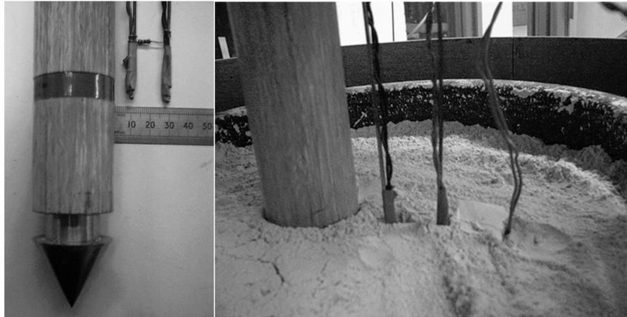
Fig. 9. Position of the thermistors relative to the heater. On the left the thermistors are shown next to the penetrator as they would appear if the target was transparent. On the right is the penetrator and thermistors deployed in the material.
