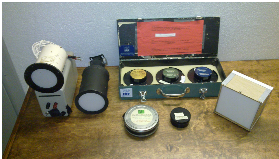
Fig. 2. Some of the low-light sources intercalibrated at this workshop. From left: IRF Lauche lamp (and powersupply), PGI Chernouss-38AM, IRF UJO-Y275, IRF UJO-L1614, IRF UJO-920B, IRF Lycksele-lamp. Front row: the Fritz Peak international standard transfer source and the MPI-2 source.
