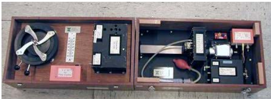
Fig. 1. The calibration photometer built by W. Barke and Hans Lauche in Lindau 1984. The source under calibration is attached to the centering device on the left. A mirror and an optical path underneath lead the light through the filter-wheel to the photomultiplier tube (PMT) on the right.
