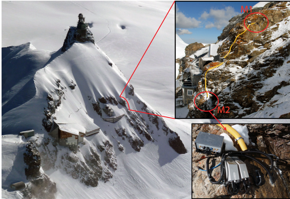
Fig. 7. Field deployment at Jungfrauoch, close-up of the measurement site and detail of measurement system M2.
