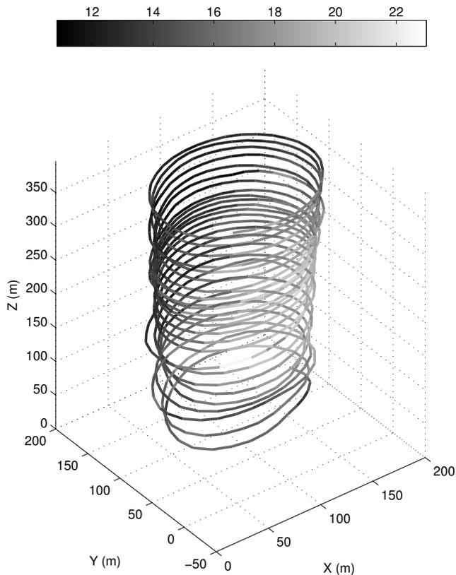
**Fig. 2.** A trace of a flight path on 17 November 2011. The shading indicates the SMARTSonde's ground relative speed ( $\text{m s}^{-1}$ ). On this day, the wind direction was northerly, becoming more easterly with height. The winds affect on the plane's speed can be seen, as the plane moved faster with a tailwind and slower with a headwind.
