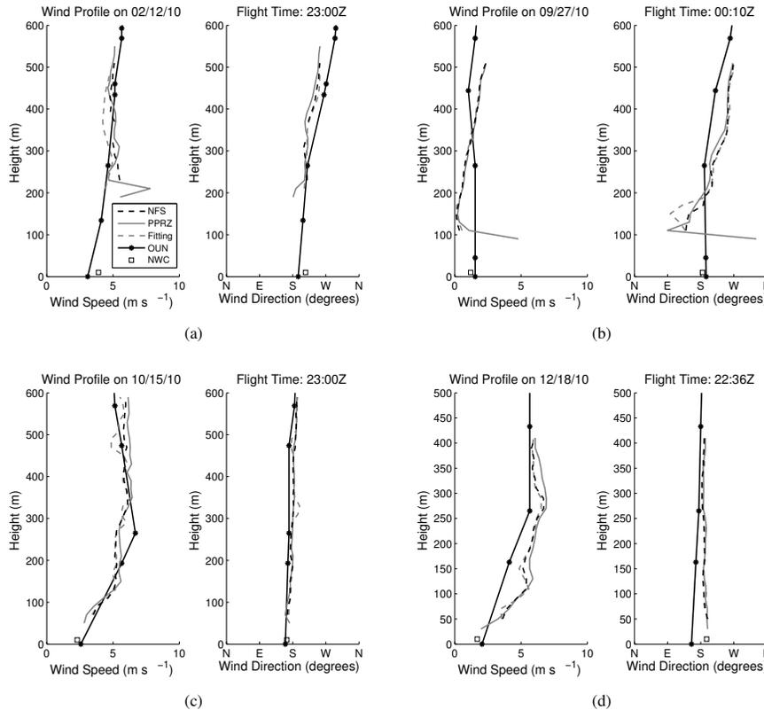
**Fig. 5.** Four examples of typical wind profiles using the different algorithms compared against the NWC Mesonet observation at 10 m (NWC, square) and the rawinsonde (OUN, solid black line with asterisks). NFS is the no-flow-sensor (dashed black line), PPRZ is the paparazzi output (solid grey line), Fitting is the best curve fitting method (dashed grey line).
