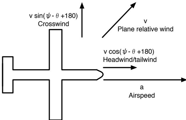
**Fig. 1.** Diagram showing the components affecting ground-relative movement of the UAS platform used in Eq. (1).
