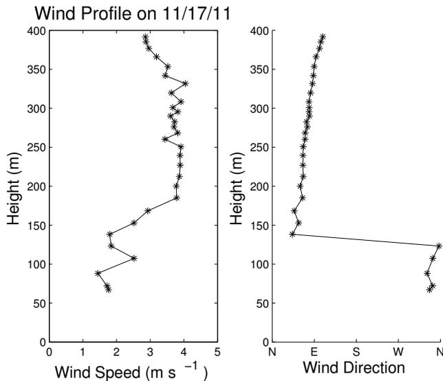
**Fig. 4.** Derived wind profile by using the best curve fitting method on the flight shown in Fig. 2.
