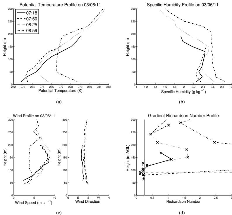
**Fig. 7.** SMARTSonde observations of the morning of 6 March 2011 from four sequential flights after sunrise. Provided is **(a)** potential temperature, **(b)** specific humidity, **(c)** wind profile using the best-curve fitting method, and **(d)** computed Richardson number. Local times for each flight is provided in the legend. Sunrise occurred at 06:53 LT.
