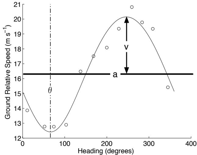
**Fig. 3.** Example fitting of the equation in the best curve fitting method. This corresponds to the circle between 207 m and 218 m above ground level (a.g.l.). The curve indicates the best fit of Eq. (1) and the circles represent the data from the GPS unit. Airspeed ( $a$ ) is marked by the solid line, wind speed ( $v$ ) is noted by the arrows, and wind direction ( $\theta$ ) is shown by the dash-dotted line.
