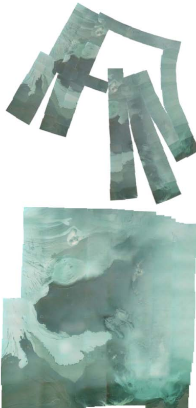
Fig. 6. Illustration of the benefits of using crossover points. Top panels: pairwise registration errors add up and lead to a huge global error. In this example, the right line of the mosaic corresponds to a featureless area, and the pairwise image registration is impacted by large errors. Bottom panels: the use of crossover points allows constraining the error. The final mosaic is consistent.
