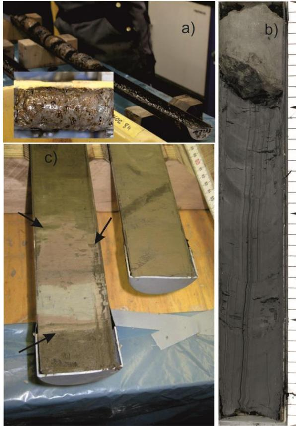
**Fig. 6.** High quality cores were drilled with MeBo from massive gas hydrate layers **(a)**, and hemipelagic muds containing authigenic carbonate precipitates **(b)** and ash layers **(c)**. Arrows point to sharp contact at the base of the ash layer and bioturbation structures at the top which are indicators of minimum disturbance of the sediments during drilling (Photos: MARUM).
