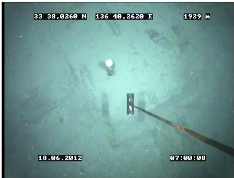
**Fig. 8.** Picture of a MeBo-CORK installed in June 2012 with MeBo off the coast of Japan. The picture was taken a few days after installation with a towed camera sled, the Ocean Floor Observation System (OFOS) of the research vessel *SONNE*. Note the imprint of the base frame and of the legs of the MeBo on the sea floor. The distance weight on a 2 m rope at the lower right of the picture belongs to the camera sled and assists the winch driver in assessing distance to sea floor (Photo: MARUM).
