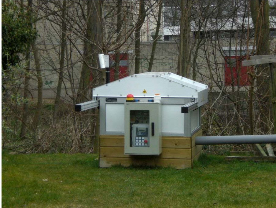
Fig. 4. Roll-off roof in real-sky test environment.
