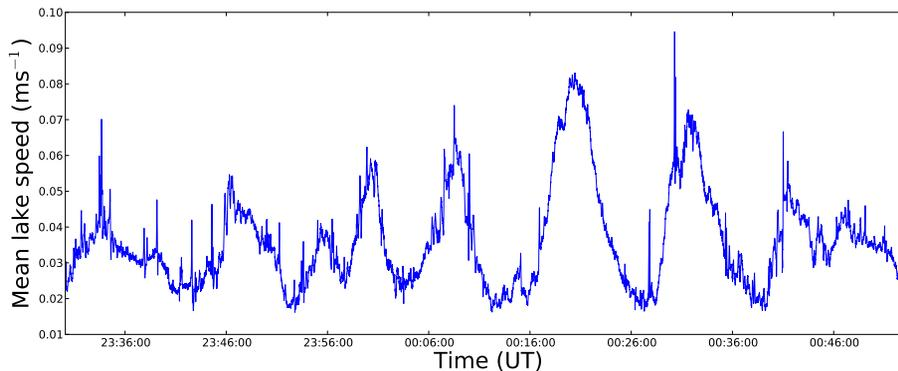
**Fig. 6.** Time series of mean lake surface speed calculated from IR images captured on 22 December 2010. The pulsatory behaviour of the lake is clearly visible with a period of  $\sim 12$  min. The sharp spikes in speed (“shot noise”) are caused by bubbles reaching the surface of the lake.
