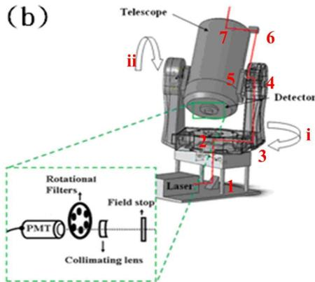
**Fig. 1. (a)** Pictorial image and **(b)** prototype model of the 3-D scanning lidar system. In figure **(b)**, the arrows *i* and *ii* show the zenith and azimuth scanning direction. Red line shows the path of the transmitting laser beam. The numbers 1 to 6 shows the position of reflection mirror. The receiver section is shown in the enlarged box in green.
