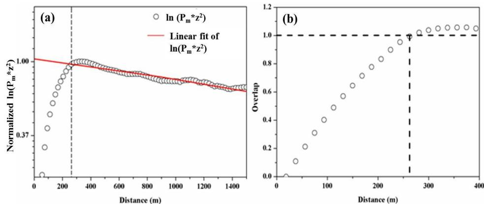
**Fig. 2.** Overlap function determination by keeping scanning lidar fixed in horizontal direction. Figure (a) shows a linear fit ( $y = -2.43 \cdot 10^{-4} \cdot x + 1.03$ , shown as a solid red line) applied to the horizontal data  $\ln(P_m \cdot z^2)$  to determine the expected signal response for the range below overlap height ( $\sim 260$  m). Figure (b) shows the resultant overlap function obtained from horizontal data  $\ln(P_m \cdot z^2)$  divided by expected signal.
