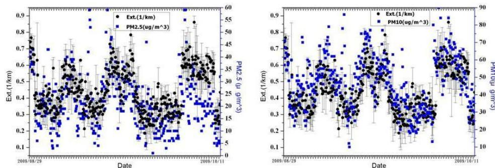
**Fig. 3.** Comparison of **(a)**  $\text{PM}_{2.5}$  and **(b)**  $\text{PM}_{10}$  concentration with the aerosol extinction coefficient derived from the scanning lidar. The PM data are hourly average; while the lidar data are shown for every 1 min. Error bars indicate the standard deviation of aerosol extinction coefficient.
