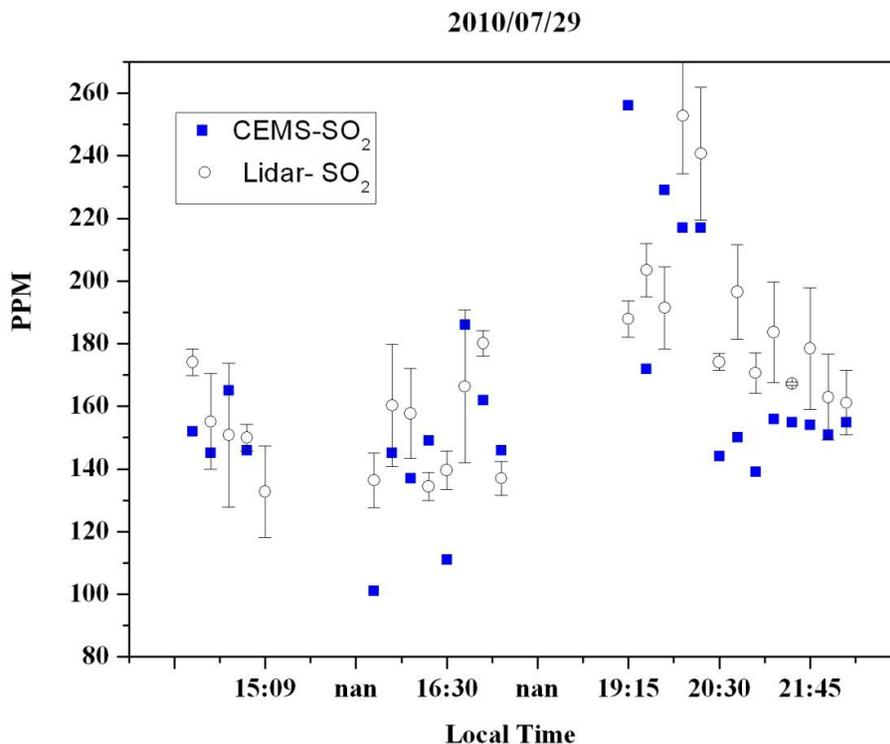
**Fig. 7.** Comparison of SO<sub>2</sub> concentration simultaneously measured from the DIAL and in-situ instruments (CEMS) on 29 July 2010. Error bars indicate the statistical SO<sub>2</sub> concentration uncertainty derived from the DIAL measurement.
