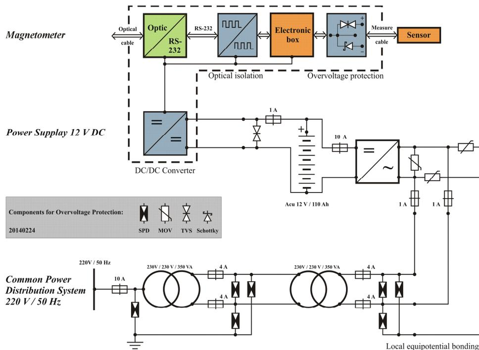
**Fig. 5.** Flow diagram of the connection of the magnetometer on the low voltage power supply network and its protection against overvoltage.
