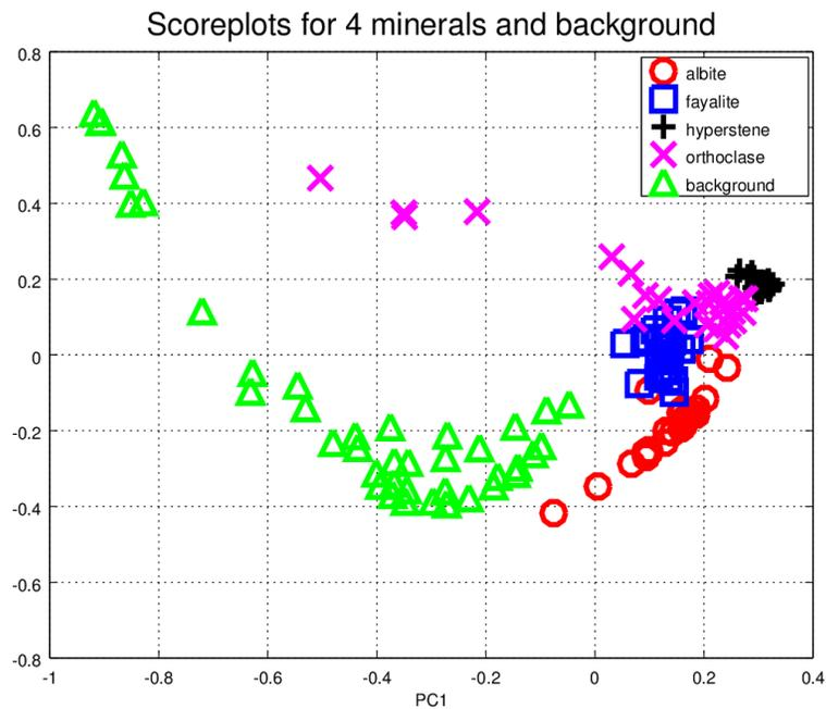
**Figure 4.** Score plot using the two first PCA components. The events represent the four minerals and the background for substrate SUB496. The scores from peak lists and RP results are essentially identical.
