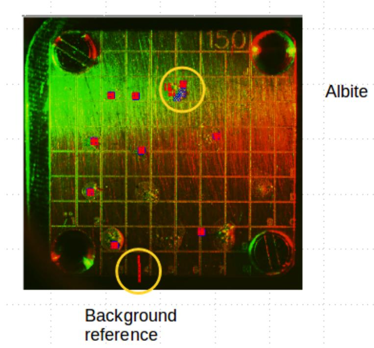
**Figure 1.** A substrate to collect dust. This one contains multiple mineral samples. In the middle at the top the albite mineral is deposited and a 5 × 5 matrix of closely spaced measurements is made. At the bottom is a straight vertical matrix of measurements on a clean area of the substrate which serves as a background reference.
