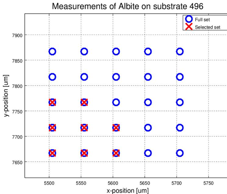
**Figure 2.** Picture showing the position of measurements at the mineral albite. The beam radius corresponds to the distance between the indicated positions. The marked squares indicate the hand picked positions on the edge of the mineral sample. As the sample is placed by wet deposition, it is likely that the other positions are contaminated by the same mineral substance in a possibly diluted form.
