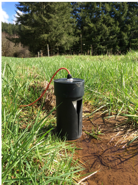
Figure 1. Field installation of water level sensor inside a flow container.
