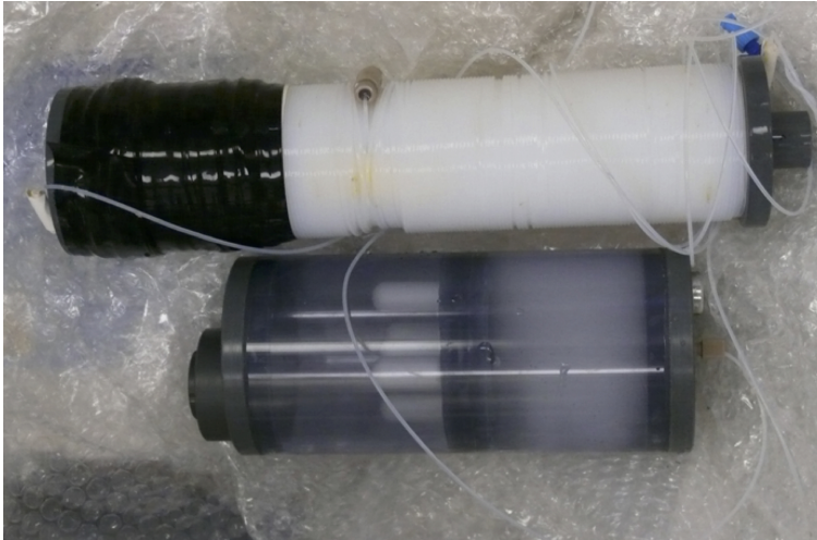
Figure 7. Osmo-sampler – tubing coil (top) and pumps (below) – that are hosted in a PVC tube attached to MeBoCORK-B.
