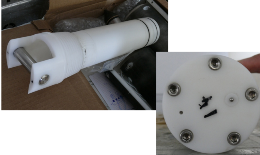
Figure 3. MeBoPlug prior to being screwed into a MeBo drill pipe (left); right photograph shows bottom view into the borehole with ports for P (hole at left) and T (little pin at right) monitoring. See text.
