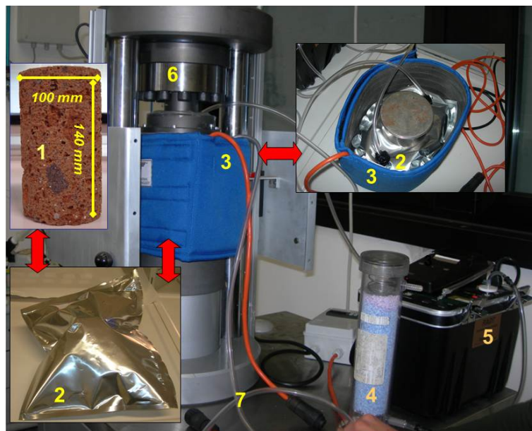
Figure 1. Experimental setup for the detection of ^{222}\text{Rn} and ^{220}\text{Rn} activity concentrations from rocks under uniaxial deformation. The system consists of: rock sample (1), DryPack accumulation chamber (2), digitally-controlled heating belt (3), desiccant (4), RAD 7 radon monitor (5), uniaxial press (6), vinyl tubing (7). Arrows connect the different sections of the experimental system to give a complete view of it. See text for explanation.
