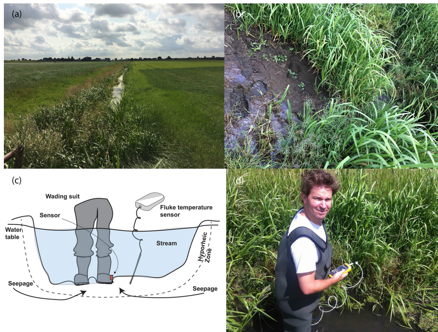
Figure 2. (a) The ditch used in the field evaluation. (b) A close-up of the boil, identifiable in the landscape by the collapsed banks of the ditch. (c) A schematic overview of the experiment during the field evaluation. (d) For scale-reference: Rolf Hut during the experiment in the ditch.
