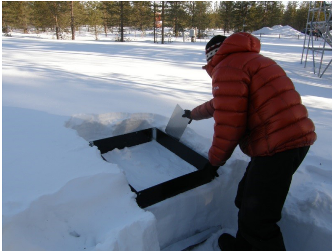
Figure 1. Snow sample was taken from snowpack with a plastic frame and a metal bottom plate surrounded by a plastic sheet.
