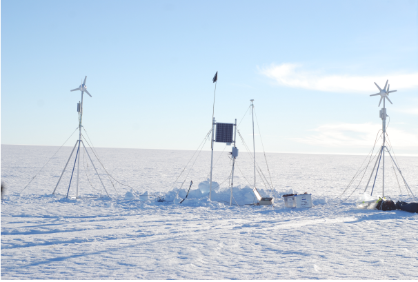
Fig. 1. GNSS station installed on the Institute Ice Stream showing the two wind turbines and solar panels required to power the GNSS receiver.
