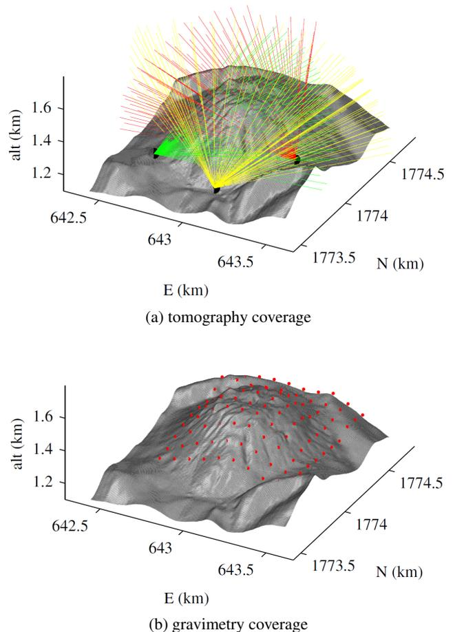
Figure 1: (a): muon tomography data coverage on the Soufrière of Guadeloupe. The lines represent the observation axes of the muon telescope when located at Rocher Fendu (red), Ravine Sud (yellow) and Savane à Mulets (green). (b): the red dots represent the positions at which we simulated gravimetry measurements
