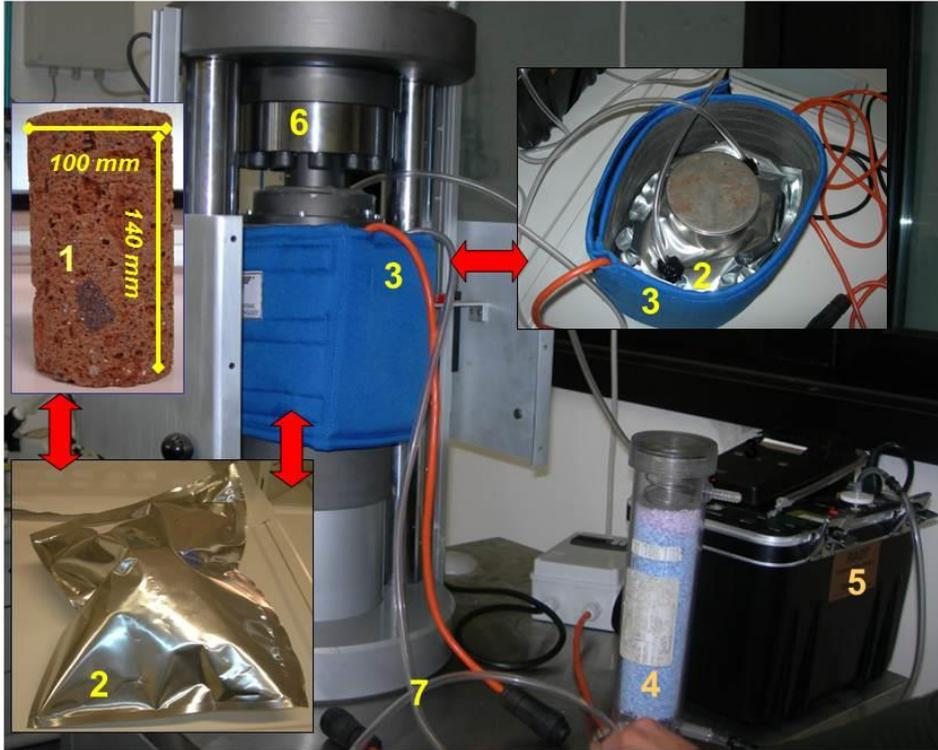
5 **Figure 1.** Experimental setup for the detection of  $^{222}\text{Rn}$  and  $^{220}\text{Rn}$  activity concentrations from rocks under uniaxial deformation. The system consists of: rock sample (1), DryPack accumulation chamber (2), digitally-controlled heating belt (3), desiccant (4), RAD 7 radon monitor (5), uniaxial press (6), vinyl tubing (7). Arrows connect the different sections of the experimental system to give a complete view of it. See text for explanation.
