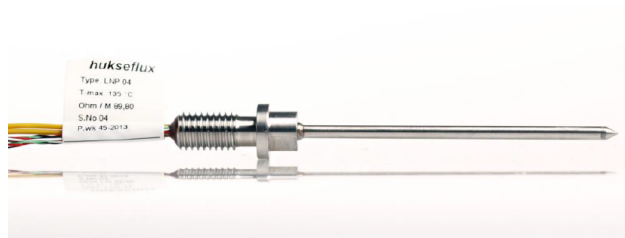
Figure 5. LNP04 thermal conductivity probe prototype. (Hukseflux, 2013)
