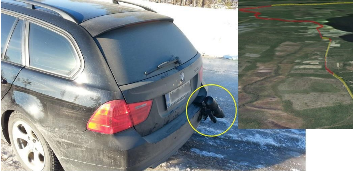
3 Figure 6. -Teconer friction measurement instrument mounted into the vehicle.
