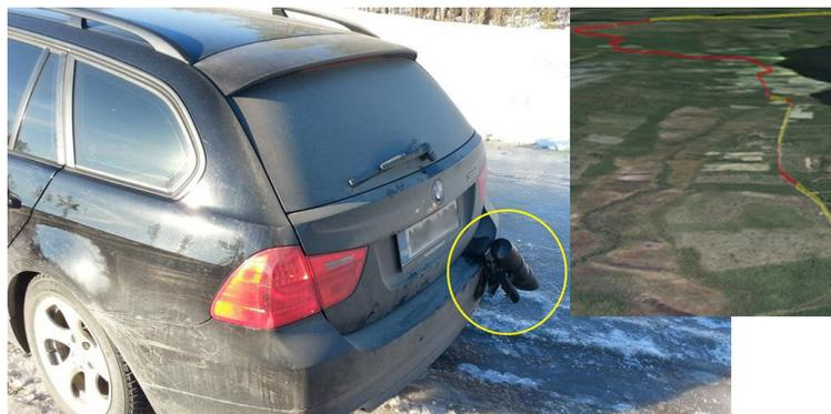
**Figure 6.** Teconer friction measurement instrument mounted into the vehicle.
