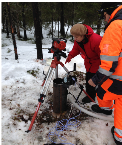
Figure 11. Installation of the Trillium Posthole 120PH seismometer in a drillcore of depth of 5.5 m at the Oulanka site (station code OLKF). Photo by Hanna Silvennoinen.
