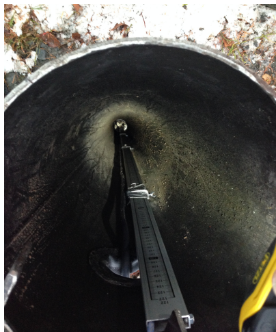
Figure 11. Installation of the Trillium Posthole 120PH seismometer in a drillcore of depth of 5.5 m at the Oulanka site (station code OLKF). Photo by Hanna Silvennoinen.
