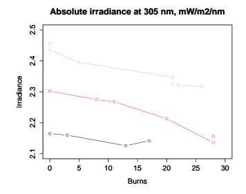
**Figure 5.** The data of Fig. 2, but plotted as a function of the number of times the lamp has been burned in darkroom calibrations. A linear fit to an exponential model suggests that the lamps fade by about 0.3 % every time they are burned.
