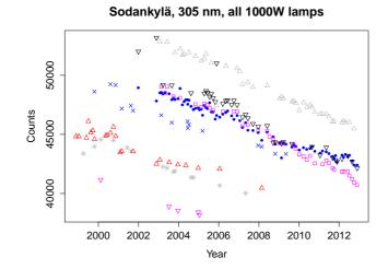
**Figure 3.** The raw counts from 1000 W standard lamp calibrations in Sodankylä up to 2013. There are no major discontinuities in the data.
