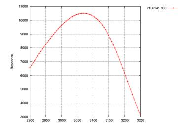
**Figure 8.** Example of a calibration. The response of the Brewer that was calculated from the measurement of the lamp d63 (Fig. 6) using the irradiance file showed in Fig. 7.
