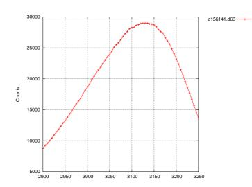
**Figure 6.** Example of a calibration. The raw spectrum for one lamp (d63) measured with the Brewer.
