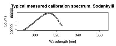
Figure 1. Typical raw outputs from a lamp calibration.
