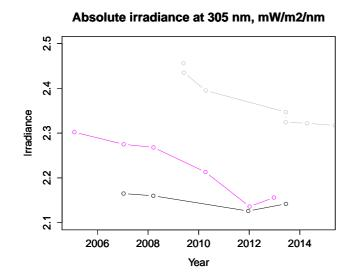
**Figure 4.** Time behavior of three primary standards that have been calibrated annually at the National Standards Laboratory MIKES-Aalto.
