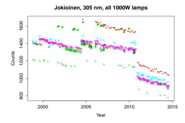
**Figure 2.** Raw counts from the calibrations of the primary and secondary 1000 W standard lamps in Jokioinen. Two discontinuities are clearly seen, during which the instrument characteristics changed significantly. In between these discontinuities, the counts fall steadily as the lamps age.
