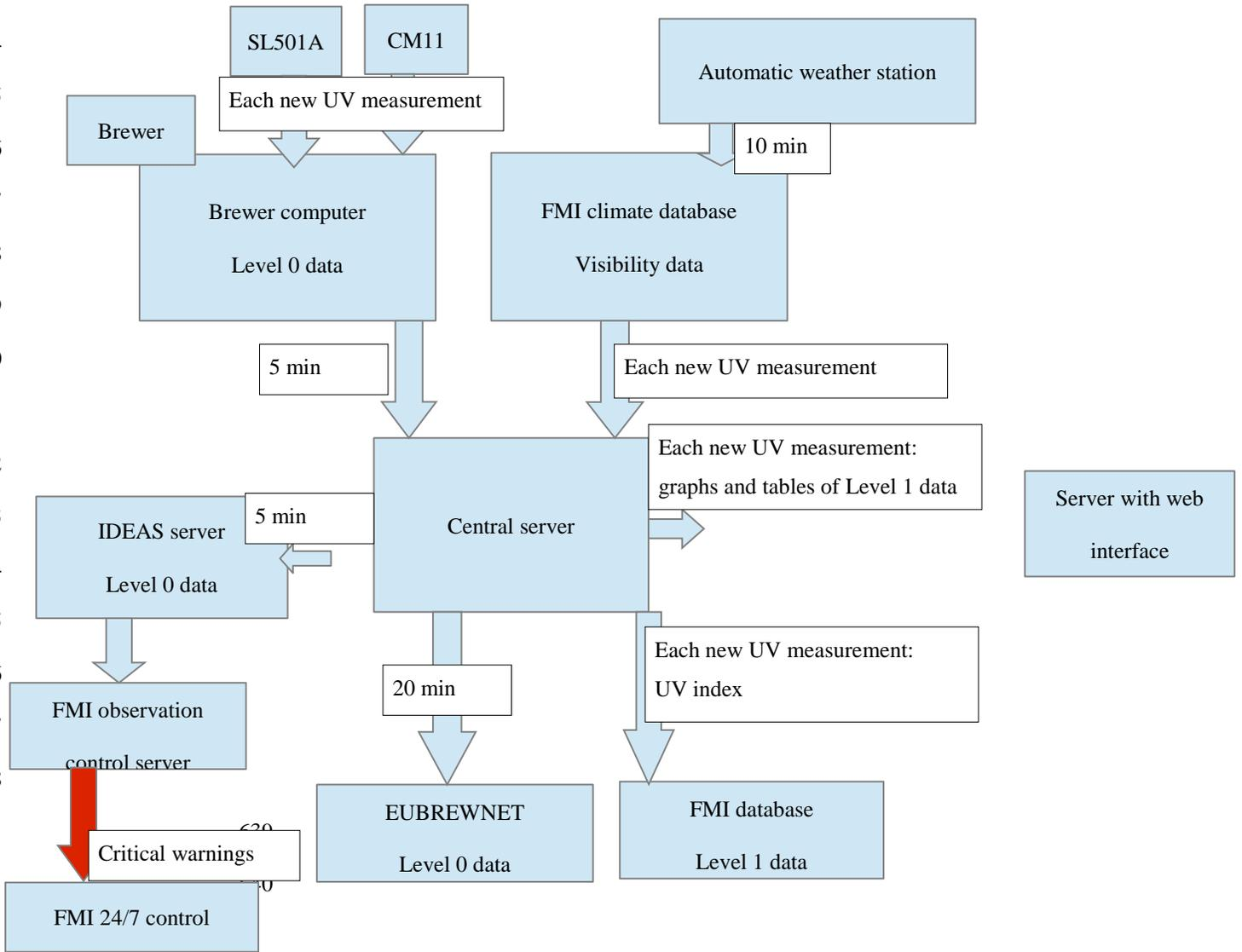
Figure 6. Schematic presentation of Brewer NRT data processing.
