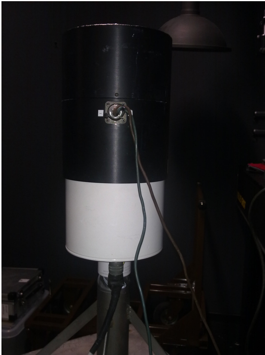
Figure 3. Lamp measurement of the NILU-UV radiometer. The NILU-UV is the white cylinder. The lamp is placed inside the black cylinder on the top of the NILU-UV.
