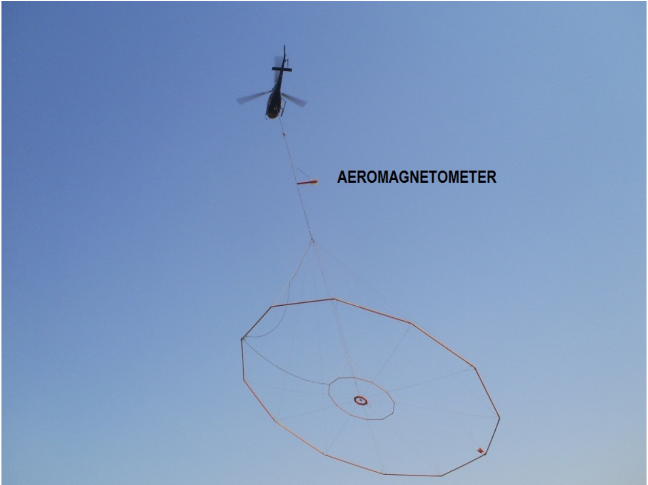
5 Figure 4 – Model of a B2 Helibras aircraft with a sensor bird and VTEM antenna. (Source: Guimarães, S. Author Private Collection, June 2008.)
