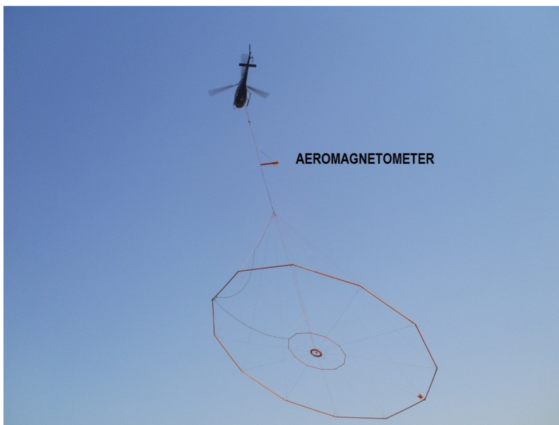
5 Figure 4 – Model of a B2 Helibras aircraft with a sensor bird and VTEM antenna. (Source: Guimarães, S. Author Private Collection, June 2008.)
