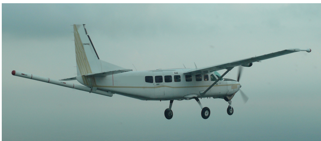
Figure 1 – Example of the C208B model geophysical acquisition aircraft. (Source: Camara, E. Author Private Collection, Sept 2014).
