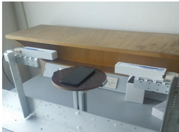
15 Fig10. Measuring setup and mobile phone used as EUT.
