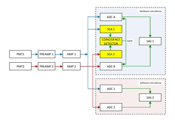
PREAMP: Preamplifier. AMP: Amplifier. SCA: Single Channel Analyzer. PMT: Photomultiplier.
