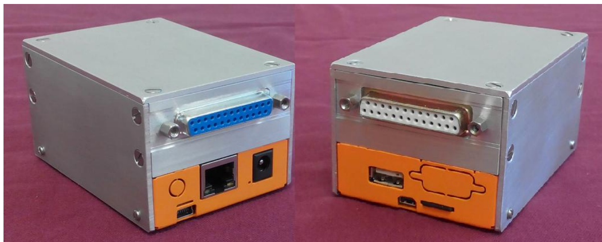
Figure 9. SAS final appearance, sized 90 mm x 60 mm x 48 mm. Both sides feature integrated connectors.
