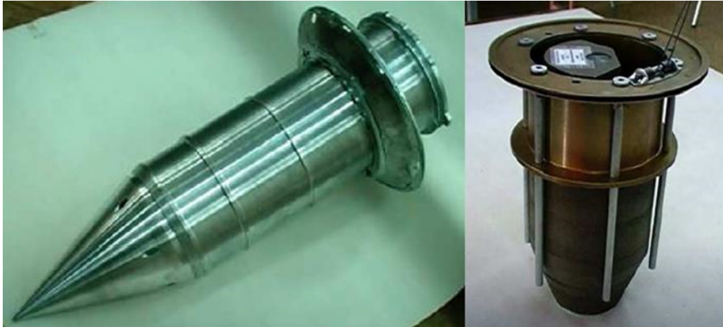
Fig. 7. On the left is shown the Surface Module forebody deployed. On the right there is the Internal Body together with Equipment Module mounted below it. Shock Absorbing System tubes are visible. The hollow tubes absorb kinetic energy by deforming as they slide through too small openings on the flanges of the Internal Body.
