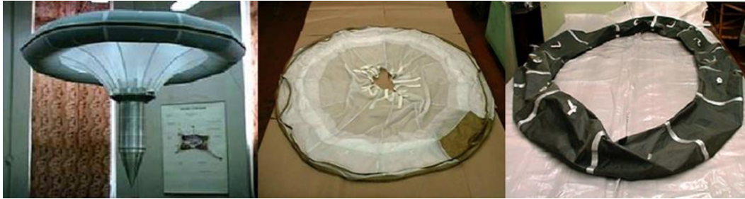
Fig. 6. Inflated Additional Inflatable Breaking Unit ( T-IBU) shown on the left with the Surface Module (SM). In the center the cover of the T-IBU and on the right the gas tight bladder.
