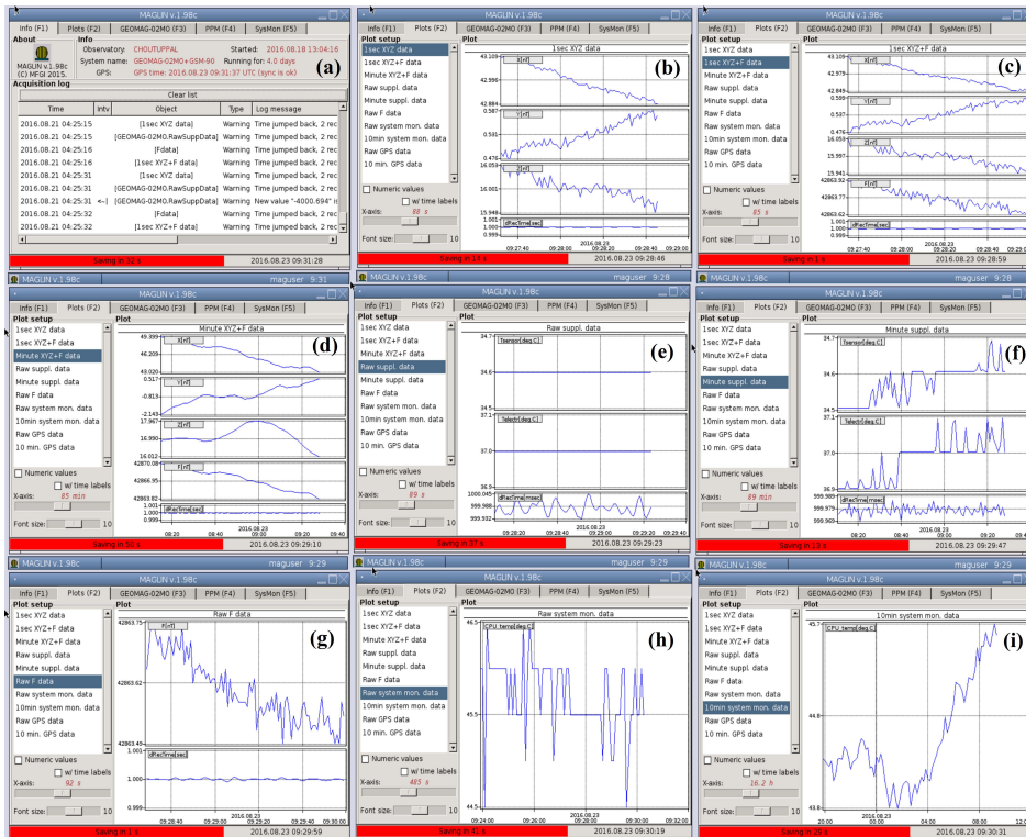
Fig. 3. Figure 06. Details of data logging and real-time plotting tools of MAGREC-4B data acquisition system
